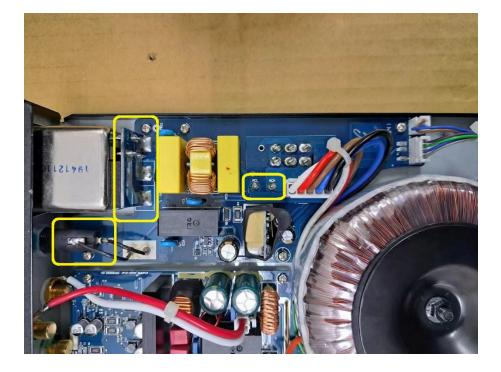
4 • Remove the screws inside the red frame
