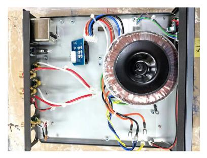
$6 \cdot \text{Replacing the circuit board of the upgrade kit}$
