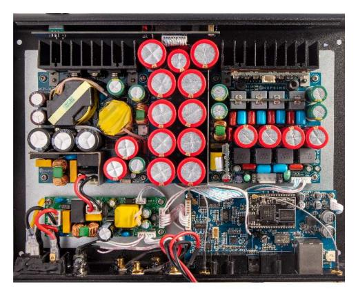
The Omnia A200 uses a compact and powerful Class D amplifier. The maximum output power can reach 250W stereo output (@4ohm speaker) and uses integrated feedback design and error correction, achieving extremely low noise and distortion. Unique Dynamic Low Noise Switching Power Supply (DLN PS) Provides excellent system-level audio performance.
