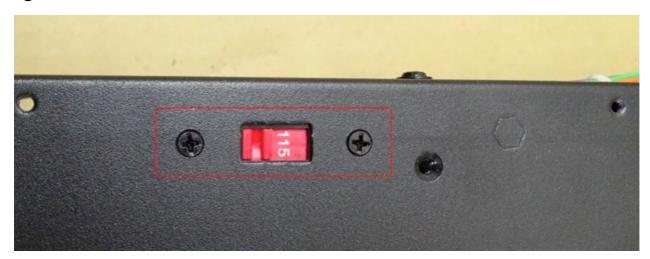
remove the 2 screws marked in red to remove the AC selector board.
