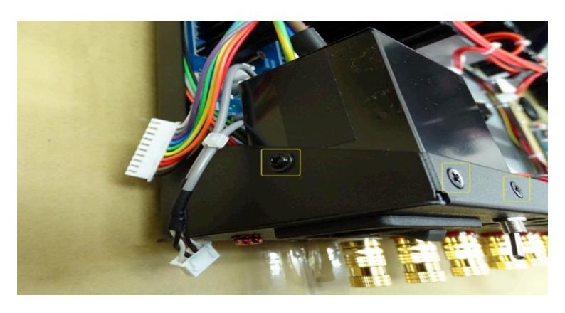
remove the 3 screws circle in yellow and move the isolation box forward to reveal the c eath.
