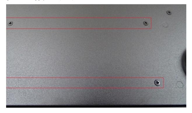
move the 4 screws from the bottom of the unit to remove the PSU.
