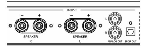
SPDIF OUT: Optical Output (up to 24 bit / 192 kHz) (No output during DSD playback)
