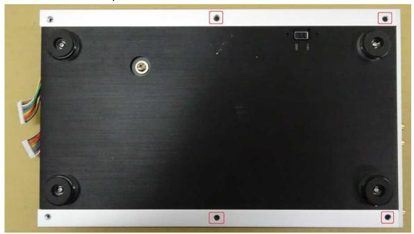
Gently slide back the top cover and install the 4 screws back to secure the cover.
