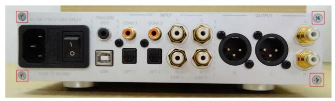
Install the 4 screws to fix the top cover and the rear panel to complete assembly.
