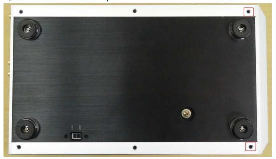
Remove the two screws marked in red on the bottom of the unit.
