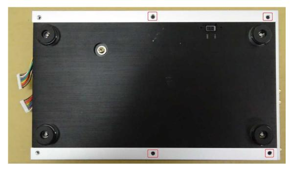
Please remove the 4 screws marked in red on the bottom of the unit. Once the screws from the rear panel and bottom unit are removed, gently pull the top cover forward to remove the top cover completely.
