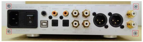
Please remove the 4 screws marked in red from the back panel.
