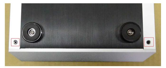
Gently slide back the front panel and install the 2 screws to secure the front panel.
