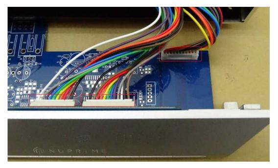
Once the screws are removed, pull out DAC-10 front panel gently to reveal the cables inside. Disconnect the cables to remove the front panel.
