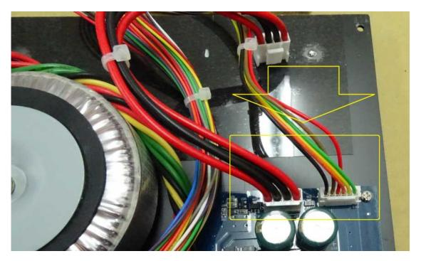
Please connected the two cables provided with the DAC-10H front panel to the main DAC board.
